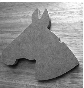
Our template will be glued onto a carrier board because it does not fully cover the clamp face. This provides stability and makes the jig easier to set up
