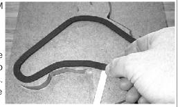
Woodworking:- Using Vac-Clamp with jigs
