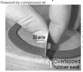
HINT To get the ends of the tape to line up, lay one piece over the other and cut through both with a sharp knife. Carefully remove the pieces that are not required and butt the two ends together
